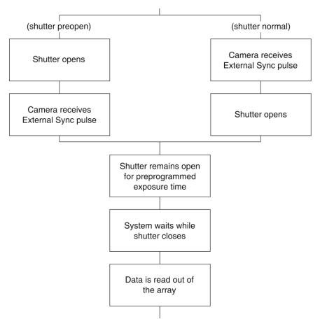
Figure 30. Chart Showing Two External Sync Timing Options
